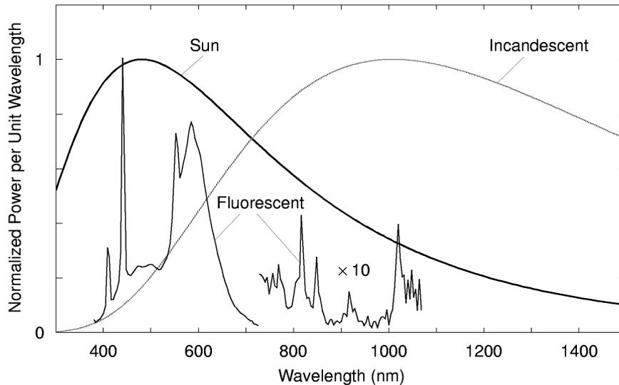
Fig. 1.3: Optical power spectra of common ambient light sources [15]
