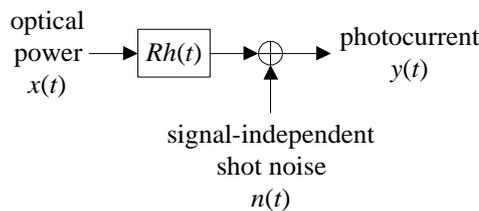
Fig. 1.1: Equivalent baseband model of an optical wireless system using IM/DD
