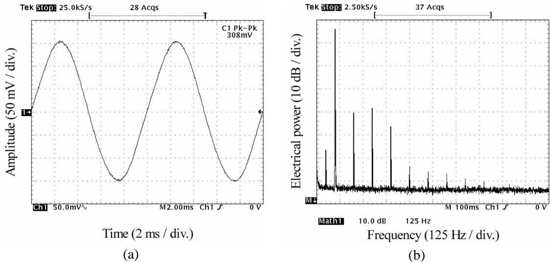
Fig. 1.4: Incandescent bulb: (a) time domain waveform, and (b) detected electrical spectrum
