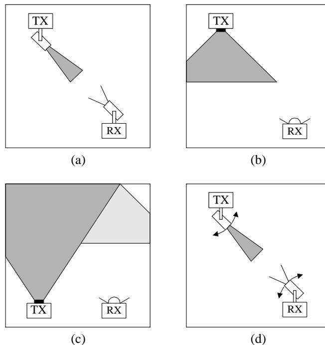
Fig. 1.2: Link configurations: (a) directed LOS, (b) non-directed LOS, (c) diffuse, and (d) tracked
